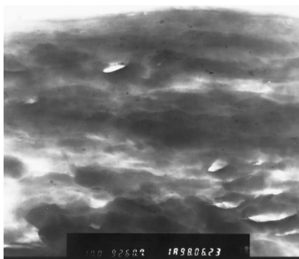
Figure 6 Axial section SEM micrograph of monofilament with 20 wt% PANI content (magnification: \times 10,000 ).
